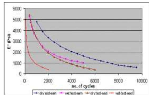
Figure-3 Dry and wet test modulus values of Brazos gravel with AAD-1 and AAM-1
