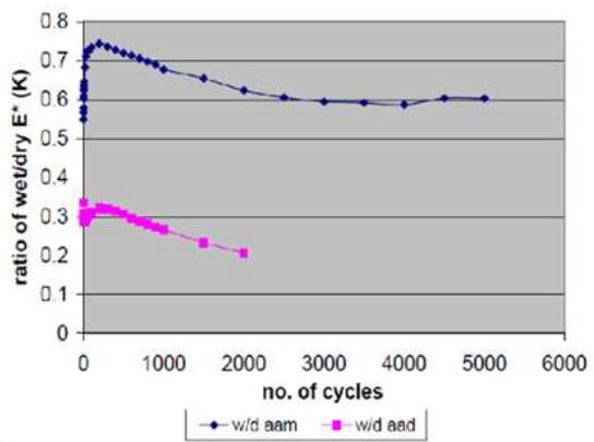
**Figure-4 Ratio (K) of wet/dry test modulus vs. no. of loading cycles for Brazos gravel**
