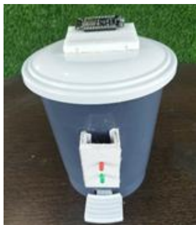
Fig 7. LED And NodeMCU ESP8266 Connected
